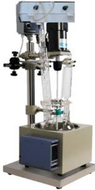
Fig. 2. External appearance of the perfusion module for extracorporeal anti-ischemic protection of the donor heart
