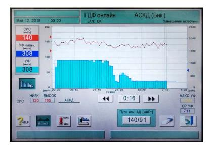
Fig. 1. An example of the automatic pressure monitoring system. The upper curve represents the systolic blood pressure level, the lower curve shows the ultrafiltration rate. There was a tendency to an intradialytic hypotension episode development in the middle of the procedure. The automatic pressure monitoring system reduced the ultrafiltration rate, thereby preventing an episode of intradialytic hypotension. On restoring
