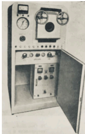
Fig. 4. TBSH-1 pressure chamber for the isolated heart preservation under increased oxygen pressure conditions [12]
